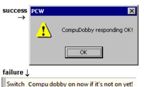
Next try the **solenoid test** (p.18). If the solenoids respond as expected, the computer is talking to the loom OK, but not receiving a reply.
